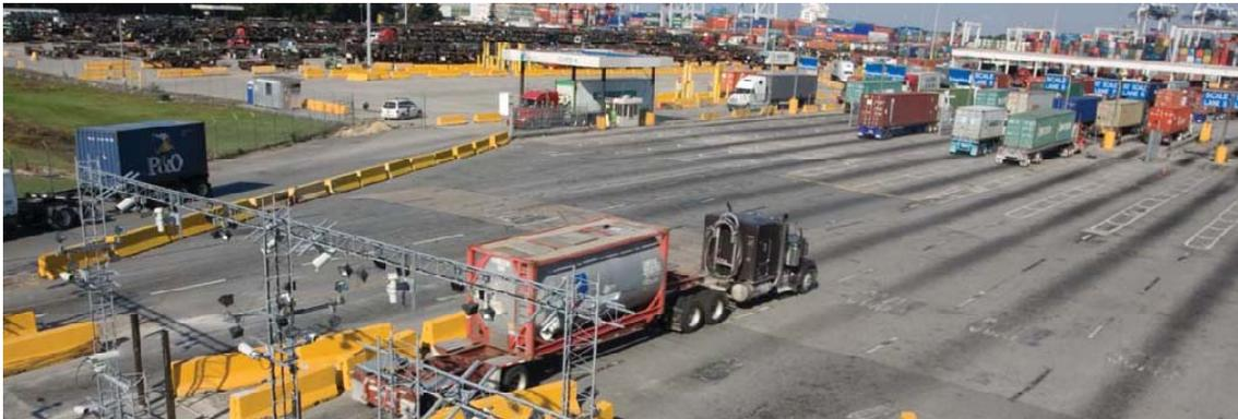
Visibility data from RFID-tagged street trucks can be used to speed processing through terminal gates
