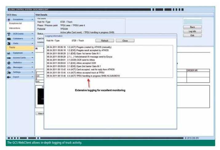
Every phase is monitored and the traceability of truck, driver and containers is easy. It merges LPR and OCR events from incoming and outgoing gates for a single truck. It gives a viewer to all images and video files captured at the OCR portals. You can also integrate nuclear detection systems, where alarms can be interfaced to route trucks if necessary.
